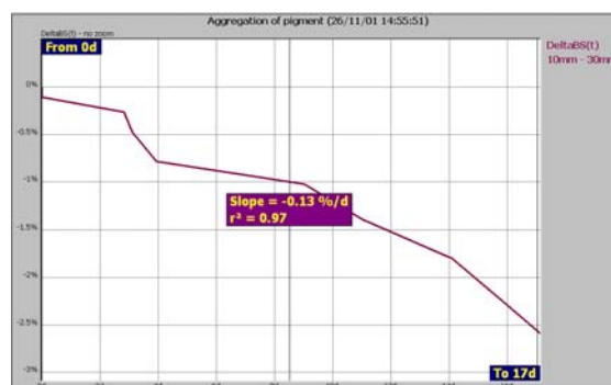
Figure 13. Variation of the backscattering (in %) as a function of time (in days).
