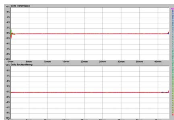
Figure 8. Transmission (top) and backscattering (bottom) for formulation 1 at 25^\circ\text{C} .
